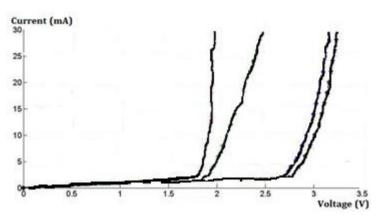
Figure 1. Current-voltage characteristic of the LED lighting system.
